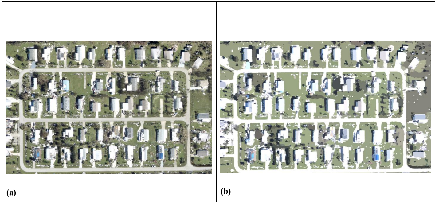
Figure 2:6 (a) Original Post-Hurricane Image, and (b) Segmented Post-Hurricane Image
